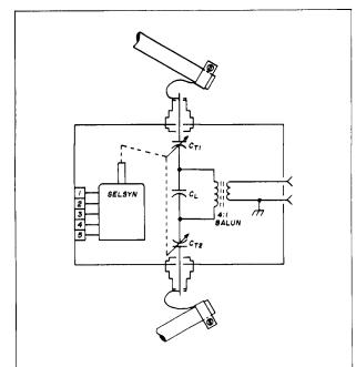
fig. 2. Simplified diagram of the contents of the control box on the boom of the antenna.
