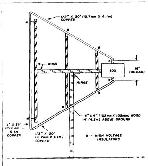
fig. 1. The structure of the SEED antenna and its mounting (not to scale).
