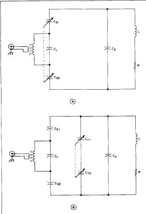
fig. 3. Circuit of the SEED antenna: (A) the elementary circuit originally envisioned, and (B) the practical circuit in use. (Component designations are explained in text.)
