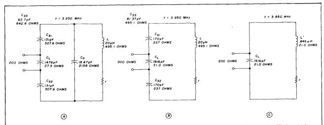
fig. 5. Transposition of the actual circuit of the SEED antenna (A); to the equivalent circuit (B); and to the simplified equivalent (C), as described in appendix B.
